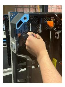
The LED module will release from its magnetic grip and become unseated. The person on the front side of the LED wall will be there to help secure the module once it has been unseated so that the person behind the LED wall can release their grip on the LED module handle.
