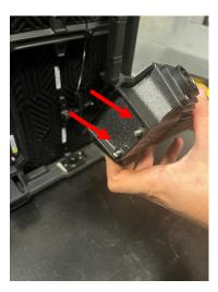
• While holding the MCU vertically, place the set pins into the receiving slots located at the bottom center of the LED panel frame.
