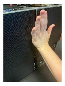
• Once you confirm that the module is flush, check the module to make sure that it does not have any damaged pixels or issues and matches the module around it. When the visual check is completed, you are finished.
