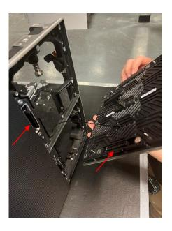
Place the lower edges of the LED module in place making sure to align them with the top edge of the LED module below.
