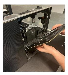
• Slowly raise the LED modules top half towards the LED panel frame. You will feel the magnetics begin to engage and guide the LED module into its correct position.
