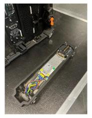
The THIRD STEP to replacing the main control unit will be to install a new MCU in place of the bad or faulty unit that was just removed.
