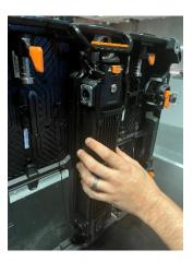
• When the top of the main control unit is near its final position, pull the latch handle up so that the latch hooks move past the latch pins on the LED panel.
