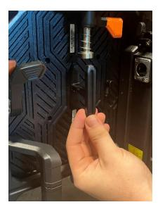
• Grip the handle with one hand and push the module towards the front of the LED wall with strong and consistent pressure.
