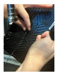
While continuing to work from the front side of the LED wall, carefully align the contact pins
