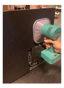
• With even and steady force pull back towards yourself to unseat the module from its magnetic holders. The module vacuum must stay on during this entire process.
