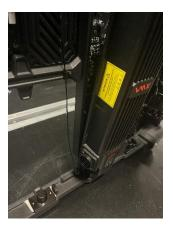
Once the set pins are securely inserted into the receiving slots, push the top of the MCU towards the top latch pins located at the top of the LED panel frame.
