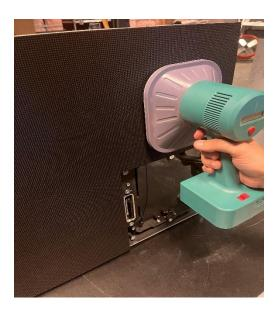
• Once your module vacuum is pressed against the LED module, turn the module vacuum to the one position. You will feel suction against the LED module.
