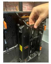
• Continue to pull upwards on the latch handle until the latch catch is no longer engaged with the latch pins.
