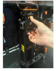
• Depress the release button with your thumb and pull the latch handle upwards with your fingers. You will see the top of the main control unit start to disconnect from the back of the
