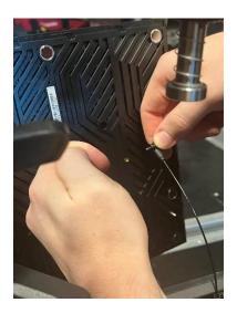
• When the module safety line is disconnected, the person on the front of the LED wall, that is holding the LED module can fully remove the LED module and put it in a safe location.
